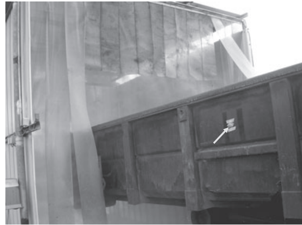
Fig. 4 Commercial disinfecting facility at work at Gan Shmuel. The arrow points on the sealed mesh bags containing Phelipanche aegyptiaca seeds placed on the container wall.
