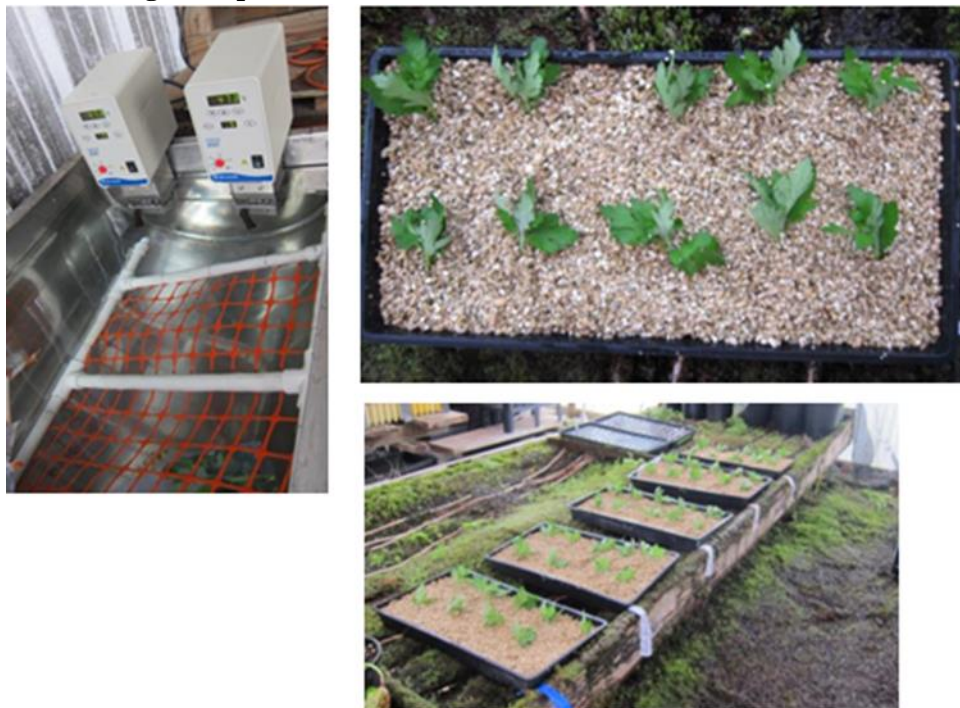
Figure 17. Two immersion heating/circulating pumps were attached to a stainless steel sink and used to achieve target temperatures.
