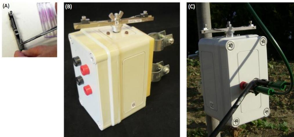
(A) Sampling rod on rotorod arms; (B) Rotorod sampler unit with arms attached; (C) Rotorod sampler unit with power cable in the field.
